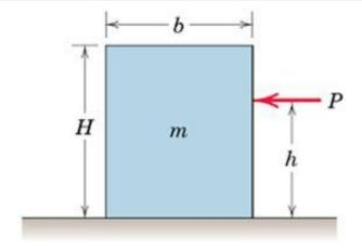
The block moves with constant velocity under the action of P.  $\mu_k$  is the Coefficient of Kinetic Friction. Determine:
