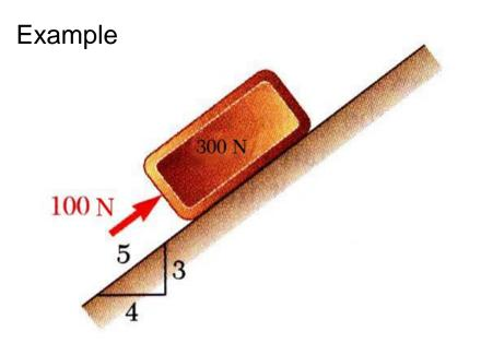
A 100 N force acts as shown on a 300 N block placed on an inclined plane. The coefficients of friction between the block and plane are  $\mu_s = 0.25$  and  $\mu_k = 0.20$ . Determine whether the block is in equilibrium and find the value of the friction force.
