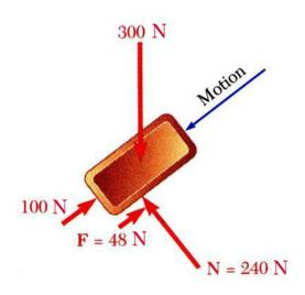
If maximum friction force is less than friction force required for equilibrium, block will slide. Calculate kinetic-friction force.
