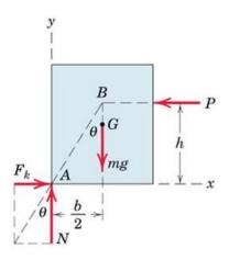
Alternatively, we can directly write from the geometry of the FBD:
