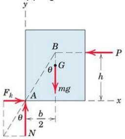
The resultant of  $F_k$  and N passes through point B through which P must also pass, since three coplanar forces in equilibrium are concurrent.
