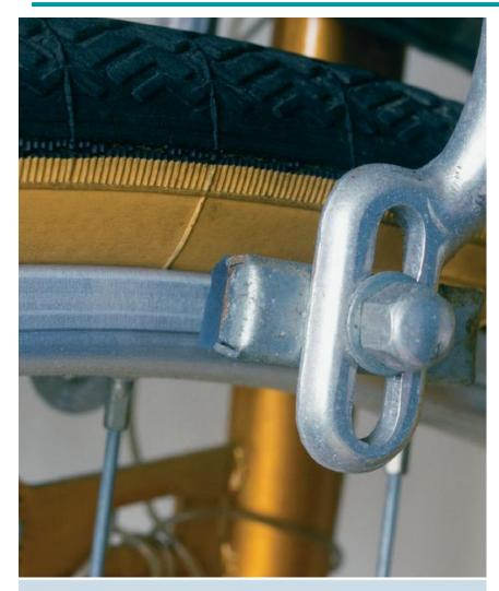
The effective design of a brake system, such as the one for this bicycle, requires an efficient capacity for the mechanism to resist frictional forces. In this chapter, we will study the nature of friction and show how these forces are considered in engineering analysis and design.
