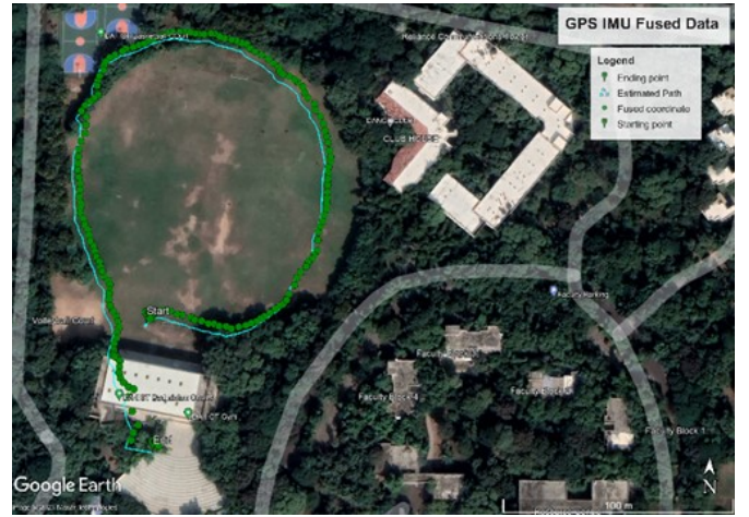
Fig. 8. IMU and GPS fused coordinates are depicted with dot (green) symbols. Solid line (light blue) indicates the estimated path obtained from KPE.
