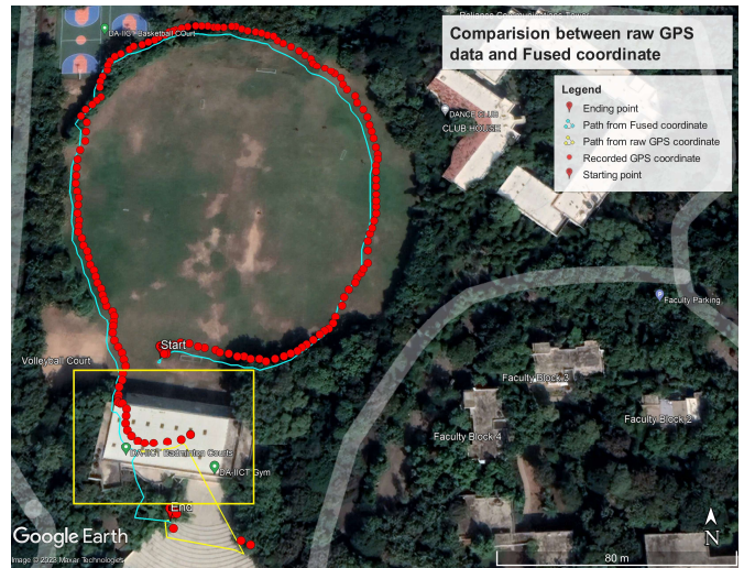
Fig. 9. Comparison of measured GPS data (depicted earlier in Fig. 4) and estimated path obtained using KPE. The yellow square box highlighted that the missing of few red points measured from GPS which results inaccurate response of GPS for indoor navigation. This inaccuracy is solved with the help of fused IMU and GPS responses.
