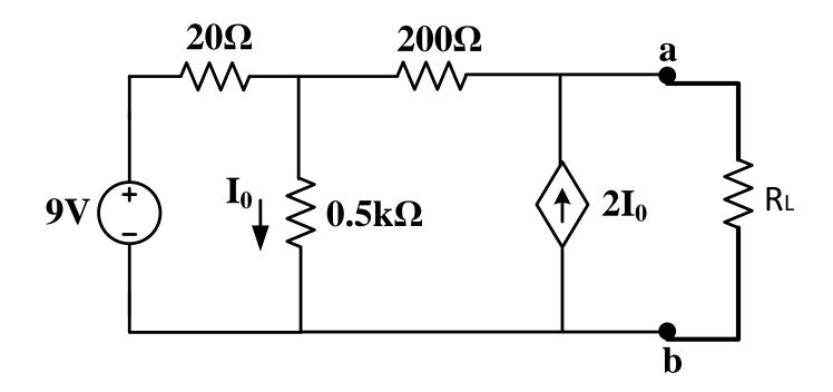
After disconnecting  $R_L$ , let the voltage across 0.5 k $\Omega$  be Vx and the open circuit voltage across **a-b** be the Thevenin's voltage Vth.
