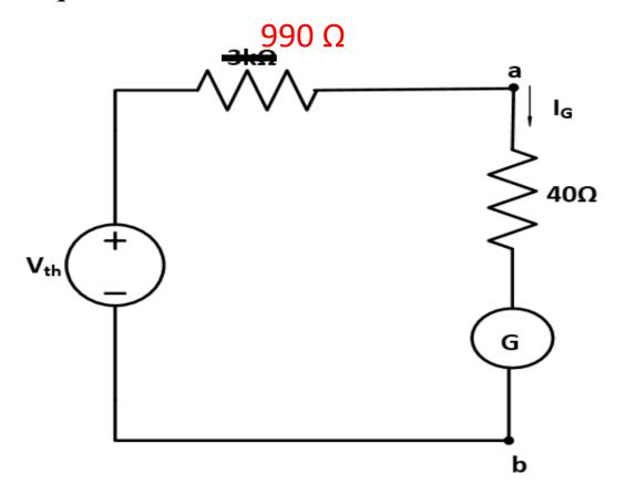
$$I_G = \frac{V_{Th}}{R_{Th} + R_m} = \frac{-77}{990 + 40} = -74.76 mA$$
