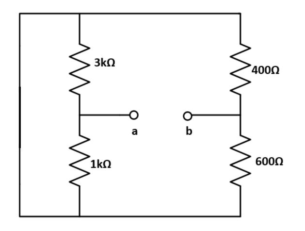
Notice that  $3 \text{ k}\Omega$  and  $1 \text{ k}\Omega$  resistors are in parallel and so are the  $400 \Omega$  and  $600 \Omega$  resistors. The two parallel combinations form a series combination with respect to terminals  $\mathbf{a}$  and  $\mathbf{b}$ .
