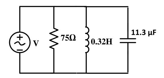
Reactive power of the capacitor,  $Qc = -V_{rms}^2/Xc = -204.04 \text{ VAR}$
