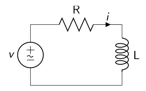
Given,  $v(t) = 240\sqrt{2}\sin(1000t) \text{ V}$ , R =  $4\Omega$  and L = 3mH
