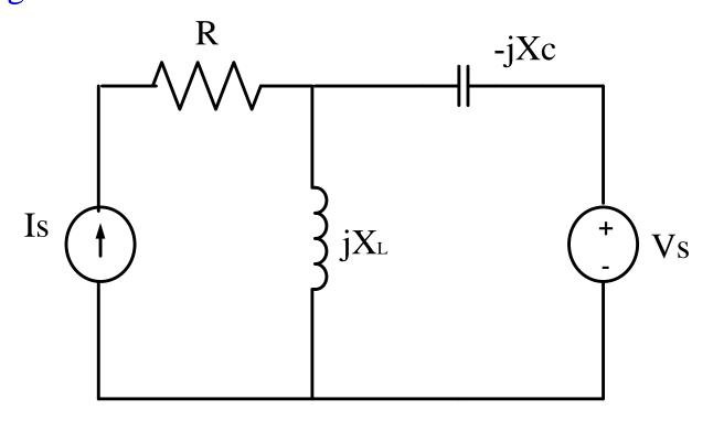
Given Is = 5 Sin wt A and  $Vs=55 \text{ Sin (wt+30^0)} V$
