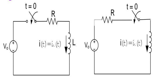
Using Source Transform DC voltage source  $V_0$  and series R can be replaced by
