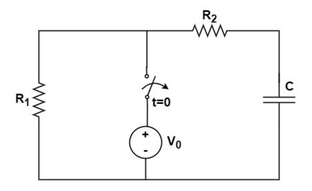
Given:  $R_1$ = 4 Ohm,  $R_2$ = 8 Ohm, C=20 microFarad and  $V_0$ = 18 V.
