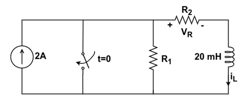
$$v_R(0^+) = 10 \text{ V and } v_R(1 \text{ ms}) = 5 \text{ V}$$
