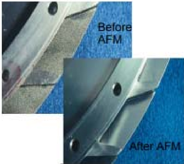
Internal passages within turbine engine diffuser
