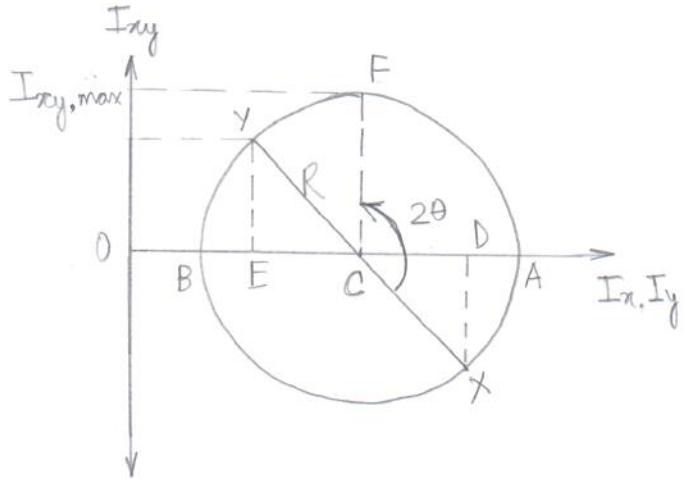
CF corresponds to the maximum product of inertia, i.e.  $I_{xy,\max}$ . Thus, the x axis lies  $2 \times 67.5^\circ$  ( $2\theta$ ) clockwise from CF.
