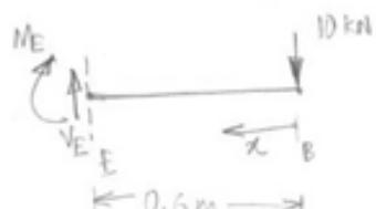
$$\sum M_B = 0 \Rightarrow -M_E - V_E \times x = 0 \\ \Rightarrow M_E = -10x \text{ kN}\cdot\text{m}$$
