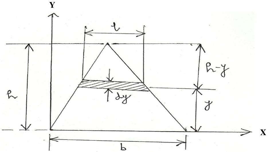
A differential strip parallel to the x axis is chosen for dA
