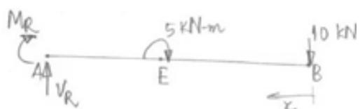
For SFD and BMD, a section of beam is isolated and free-body diagram is shown as
