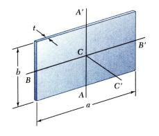
• For the principal centroidal axes on a rectangular plate,  $I_{AA'} = \rho t I_{AA',area} = \rho t \left(\frac{1}{12}a^3b\right) = \frac{1}{12}ma^2$   $I_{BB'} = \rho t I_{BB',area} = \rho t \left(\frac{1}{12}ab^3\right) = \frac{1}{12}mb^2$   $I_{CC'} = I_{AA',mass} + I_{BB',mass} = \frac{1}{12}m(a^2 + b^2)$
