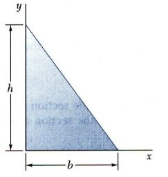
Determine the product of inertia of the right triangle (a) with respect to the x and y axes and (b) with respect to centroidal axes parallel to the x and y axes.
