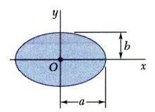
Moment of inertia about x-axis $I_x = \frac{1}{4}\pi ab^3$ Moment of inertia about y-axis $I_y = \frac{1}{4}\pi a^3 b$
