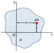
• Product of Inertia of area A w.r.t. x-y axes:  $I_{xy} = \int xy \, dA$
