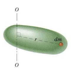
Consider a three dimensional body of mass *m* Mass moment of inertia of this body about axis *O*-*O*:
