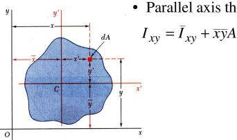
• Parallel axis theorem for products of inertia:
