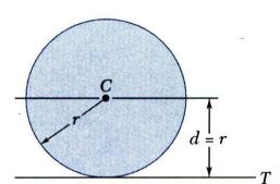
• Moment of inertia  $I_T$  of a circular area with respect to a tangent to the circle,
