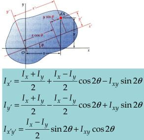
Adding first two eqns:  $I_{x'} + I_{y'} = I_x + I_y = I_z \rightarrow$  The Polar MI @ O
