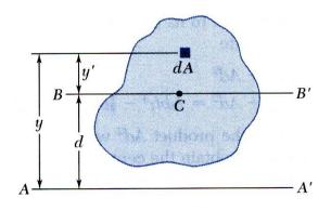
Parallel Axis theorem: MI @ any axis = MI @ centroidal axis + Ad<sup>2</sup>
