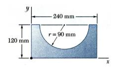
• The moment of inertia of the shaded area is obtained by subtracting the moment of inertia of the half-circle from the moment of inertia of the rectangle.
