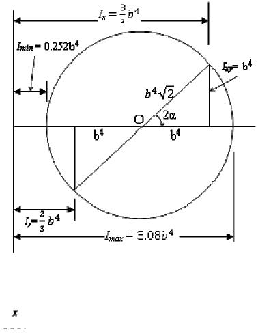
Q. No. Determine the moments and product of inertia of the area of the square with respect to the x'- y' axes.
