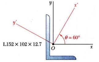
The moments and product of inertia with respect to the x and y axes are  $I_x =$ 7.24x106 mm<sup>4</sup>,  $I_y = 2.61x106$  mm<sup>4</sup>, and  $I_{xy} = -2.54x10^6$  mm<sup>4</sup>.
