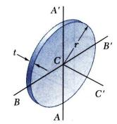
• For centroidal axes on a circular plate,
