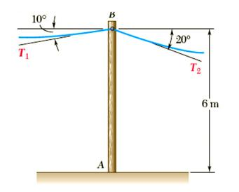
A 6-m telephone pole of 1600-N used to support the wires. Wires  $T_1 = 600$  N and  $T_2 = 375$  N.
