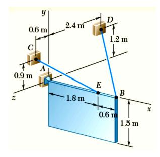
A sign of uniform density weighs 1200-N and is supported by a balland-socket joint at A and by two cables.
