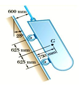
A loading car is at rest on an inclined track. The gross weight of the car and its load is 25 kN, and it is applied at G. The cart is held in position by the cable.
