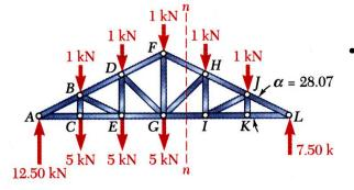
• Pass a section through members FH, GH, and GI and take the right-hand section as a free body.
