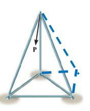
A space truss formed in this way is called a Simple Space Truss
