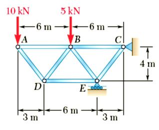
Using the method of joints, determine the force in each member of the truss.
