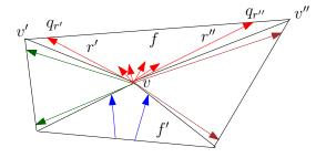
initiate a discrete wavefront from v when blue ray bundle strikes v while exploiting the non-crossing property of shortest paths
