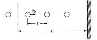
$$\Delta p = \frac{L}{l} mv_0. \quad \Delta t = \frac{L}{v_0} \cdot F_{av} = \frac{\Delta p}{\Delta t} = \frac{m}{l} v_0^2.$$
