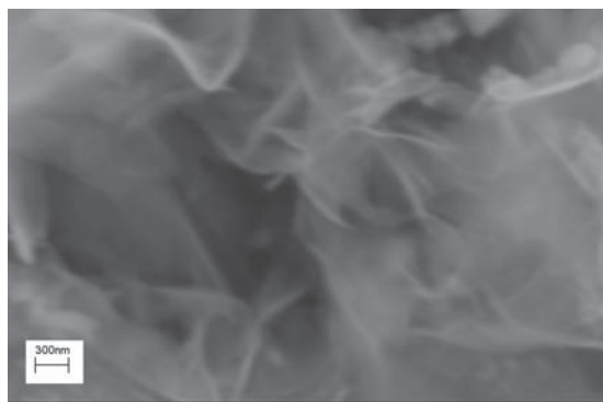
Fig. 2. SEM image of as-synthesized graphene sheets.
