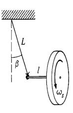
7.3 A gyroscope wheel is at one end of an axle of length l. The other end of the axle is suspended from a string of length L. The wheel is set into motion so that it executes uniform precession in the horizontal plane. The wheel has mass M and moment of inertia about its center of mass  $I_0$ . Its spin angular velocity is  $\omega_s$ . Neglect the mass of the shaft and of the string.
