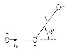
6.38 A rigid massless rod of length L joins two particles each of mass m. The rod lies on a frictionless table, and is struck by a particle of mass m and velocity  $v_0$ , moving as shown. After the collision, the projectile moves straight back.
