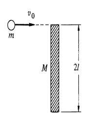
6.37 a. A plank of length 2l and mass M lies on a frictionless plane. A ball of mass m and speed  $v_0$  strikes its end as shown. Find the final velocity of the ball,  $v_f$ , assuming that mechanical energy is conserved and that  $v_f$  is along the original line of motion.
