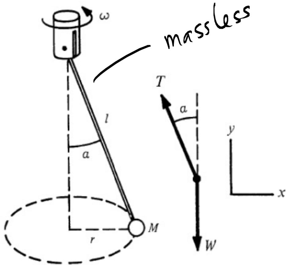
mass moves with steady speed in a circular path of constant radius!
