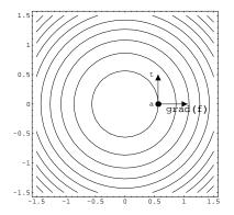
Along the tangent direction to a level curve, directional derivative must be 0! Function value does not change in that direction. But then
