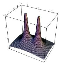
Two identical point charges at (1,0,0) and (-1,0,0). The potential in xy-plane
