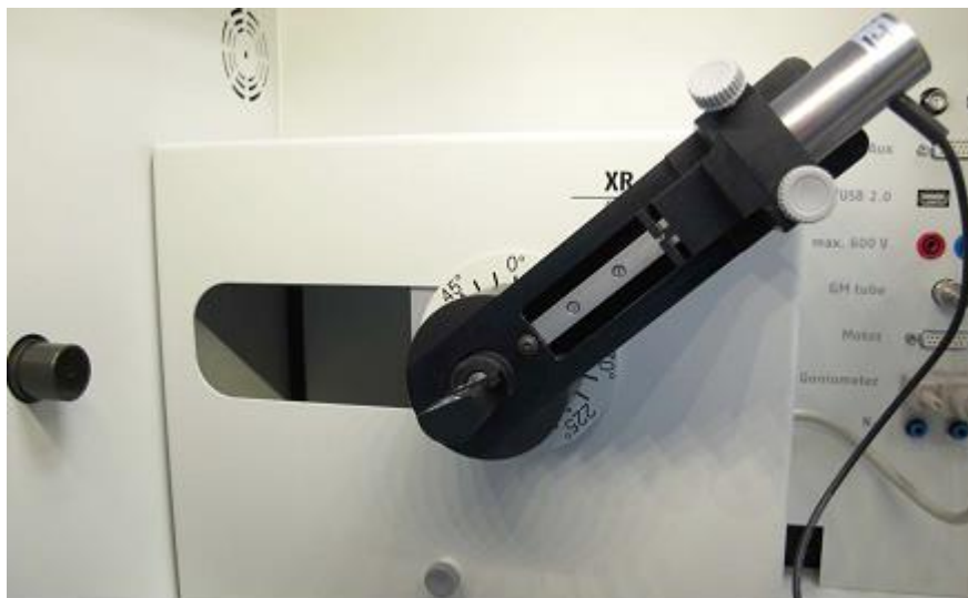
Fig. 5.1: Diaphragm and the goniometer setup
