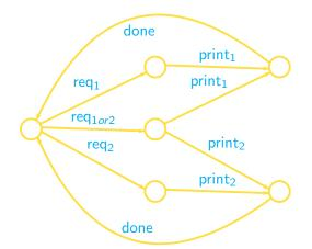
Printer 1 is colour printer, Printer 2 is black and white Schedule jobs to minimize cost — respond to  $req_{1or2}$  with print<sub>2</sub> req<sub>1</sub> print<sub>1</sub> done  $req_{1or2}$  print<sub>1</sub> done  $req_{1or2}$  print<sub>2</sub> done ... is bad req<sub>1</sub> print<sub>1</sub> done  $req_{1or2}$  print<sub>2</sub> done  $req_{1or2}$  print<sub>2</sub> done ... is OK
