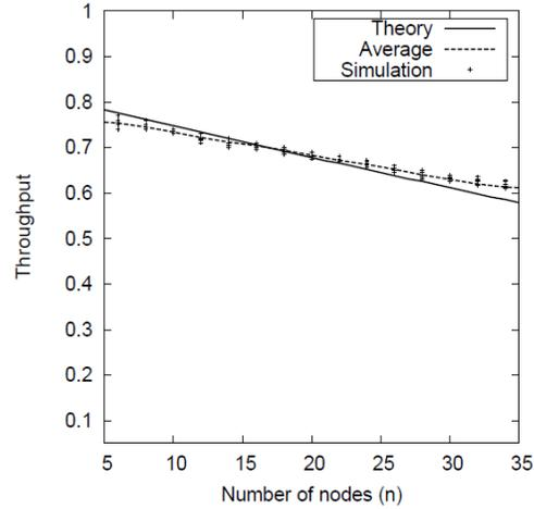
Fig. 6. Throughput of 802.11 PSM with different node size
