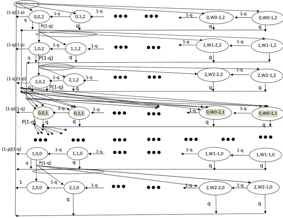
Fig. 2. Markov Model for ATIM frame transmission
