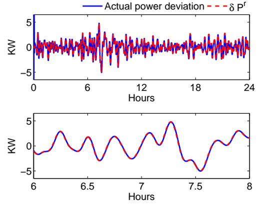
Fig. 2. Power deviation tracking performance. The 2nd plot is a 2-hour close-up.
