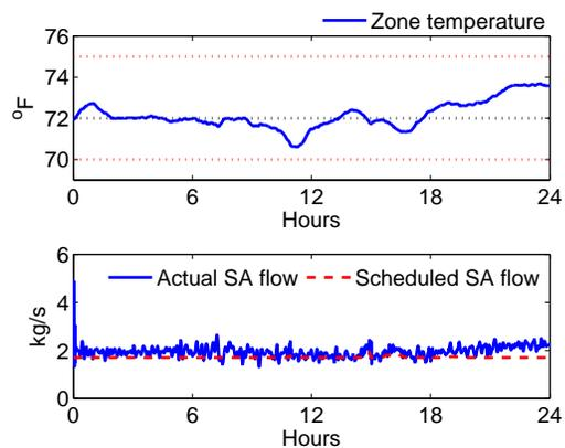
Fig. 3. Room temperature and supply air (SA) flow rate during the simulation. The red horizontal lines in top figure indicate the comfortable temperature range. The black horizontal line in top figure indicates the temperature set-point.
