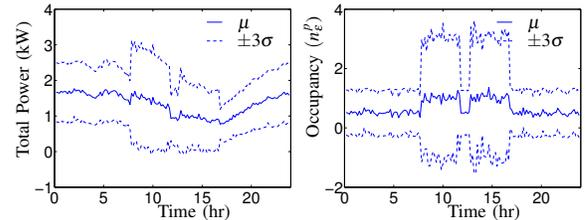
Fig. 8. Mean ( $\mu$ ) and variation ( $\pm 3\sigma$ ) of the total power (kW) and occupancy during the summer, when the outside temperature is 29.44°C and solar load is present.
