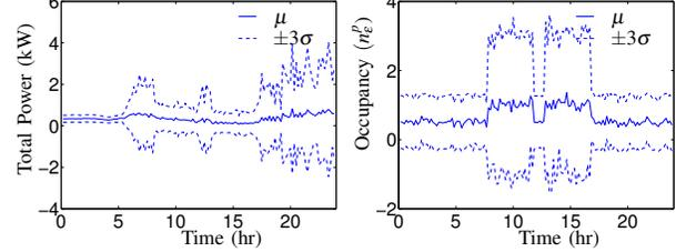
Fig. 6. Mean ( $\mu$ ) and variation ( $\pm 3\sigma$ ) of the total power (kW) and occupancy during the winter, when the outside temperature is 15.56°C and no solar radiation is present.
