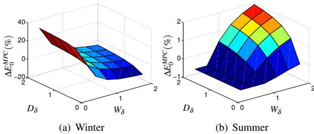
Fig. 9. Percentage change in the total energy consumption ( $\Delta E_0^{MPC}$ ) in a day as a function of parameter variation during the a) Winter, and b) Summer.
