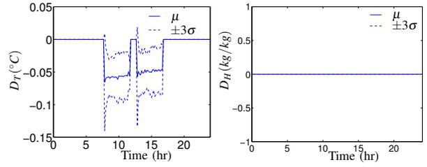
Fig. 5. Mean ( $\mu$ ) and variation ( $\pm 3\sigma$ ) of the temperature discomfort ( $D_T$ ) and humidity discomfort ( $D_H$ ) during the winter, when the outside temperature is 15.56°C and no solar radiation is present.
