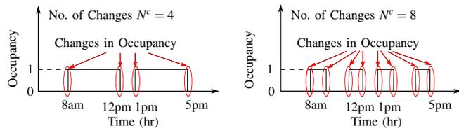
Fig. 3. Multiple occupancy profiles for fixed occupied time and different no. of changes ( $N^c$ ).
