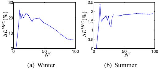
Fig. 4. Percentage change ( $\Delta E^{MPC}$ ) in energy consumption as a function of the number of the changes in the occupancy ( $N^c$ ) during the a) Winter, and b) Summer day, where the total occupancy time period is 8hrs.
