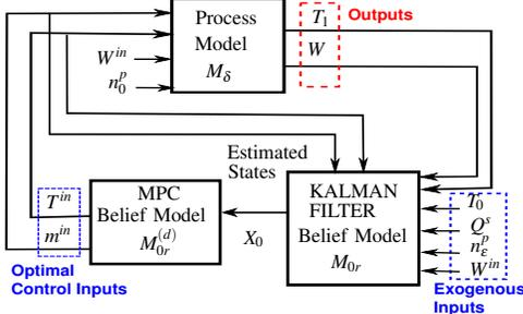
Fig. 2. Block diagram of MPC implementation for a zone-level control.
