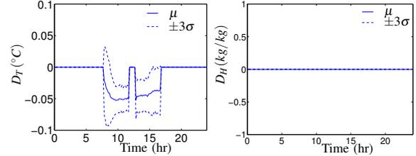
Fig. 7. Mean ( $\mu$ ) and variation ( $\pm 3\sigma$ ) of the temperature discomfort ( $D_T$ ) and humidity discomfort ( $D_H$ ) during the summer, when the outside temperature is 29.44°C and solar load is present.
