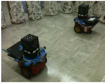
Fig. 3. Two Pioneer P3-DX robots equipped cameras and targets. Robot 1 is shown on the left, while robot 2 is on the right.
