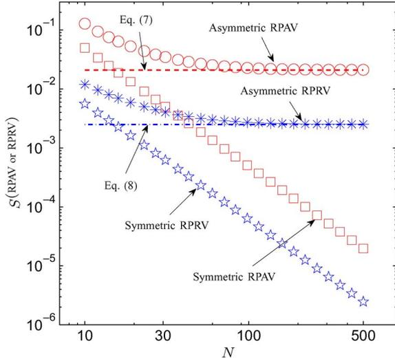
Fig. 2. Stability margin comparisons between symmetric control and asymmetric control.
