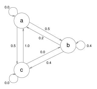
Fig. 1. Transition probability diagram for the simplified first order markov model.
