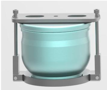
1. → Grinding bowls with standard lids have to be filled in a glove box with an inert gas atmosphere and closed using the additional clamping system. Using this procedure you can even grind hazardous substances!
