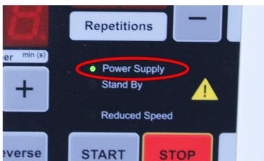
3. ➔ If POWER SUPPLY is flashing, the device is in setup mode. If POWER SUPPLY is not flashing, repeat the procedure.
