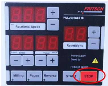
1. ➤ Press and hold the STOP button on the front of the control panel.
