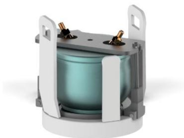
6. → Place the additional clamping system with clamped bowl in the grinding bowl holder.
