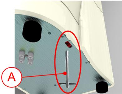
1. ➔ Insert the included triangular key (A) into the bore hole on the bottom side of the PULVERISETTE 6 *classic line* and turn it clockwise 180 degrees.
