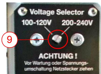
1. → Disconnect the device from the mains!
