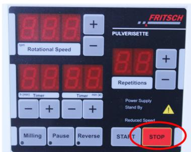
5. ➤ To save and end setup mode, press the STOP button.
