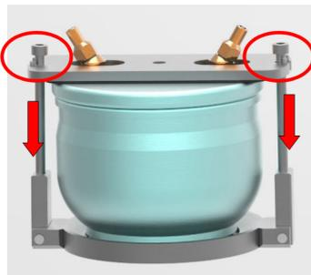
5. → Then tighten both socket-head screws (d) shown in the diagram equally with a hex key and thereby clamp the pressure plate tightly. Ensure that the pressure plate is lying evenly on the bowl lid.
