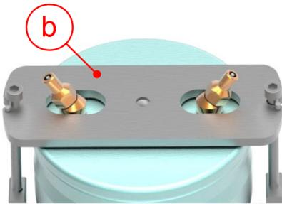
3. → Position the pressure plate (b) with the rubber disk on the bowl as shown in the picture.
