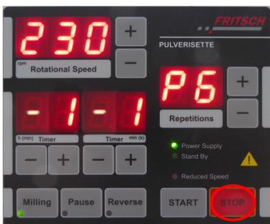
5. ➔ To save and end setup mode, press the STOP button.
