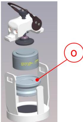
1. ➔ Place the reducer (o) (order no. 90.1120.09) into the grinding bowl holder and position the 80ml grinding bowl on it and fasten with the Safe-Lock tensioning device.
