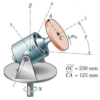
The rotor and disk have two components of angular velocity :  $\omega_0 = 120(2\pi)/60 = 4\pi$  rad/s about the z-axis and  $\Omega = 60(2\pi)/60 = 2\pi$  rad/s about the Z-axis.
