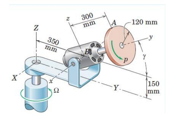
**Solution.** The rotating reference axes *x*-*y*-*z* are attached to the motor housing, and the rotating base for the motor has the momentary orientation shown with respect to the fixed axes *X*-*Y*-*Z*. We will use both *X*-*Y*-*Z* components with unit vectors **I**, **J**, **K** and *x*-*y*-*z* components with unit vectors **i**, **j**, **k**. The angular velocity of the *x*-*y*-*z* axes becomes  $\Omega = \Omega \mathbf{K} = 3\mathbf{K}$  rad/s.
