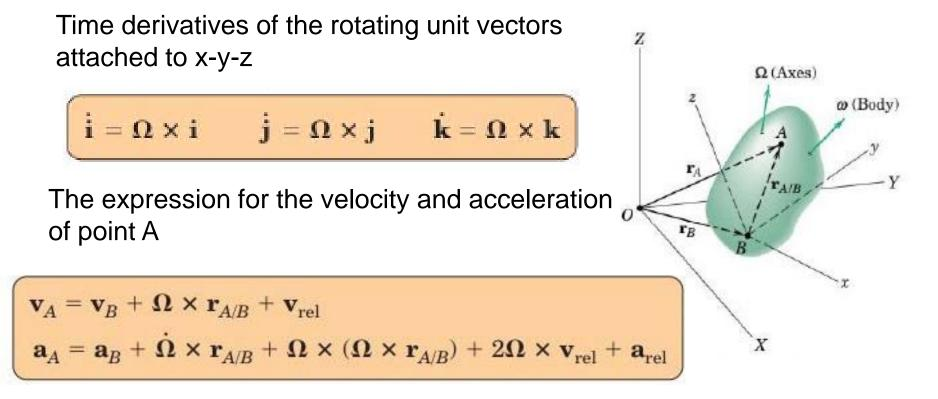
where  $\mathbf{v}_{rel} = \dot{x}\mathbf{i} + \dot{y}\mathbf{j} + \dot{z}\mathbf{k}$  and  $\mathbf{a}_{rel} = \ddot{x}\mathbf{i} + \ddot{y}\mathbf{j} + \ddot{z}\mathbf{k}$  are, respectively, the velocity and acceleration of point *A* measured relative to *x*-*y*-*z* by an observer attached to *x*-*v*-*z*.
