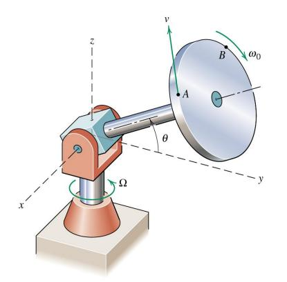
**7/7** The rotor *B* spins about its inclined axis *OA* at the speed  $N_1 = 200$  rev/min, where  $\beta = 30^{\circ}$ . Simultaneously, the assembly rotates about the vertical *z*-axis at the rate  $N_2$ . If the total angular velocity of the rotor has a magnitude of 40 rad/s, determine  $N_2$ .
