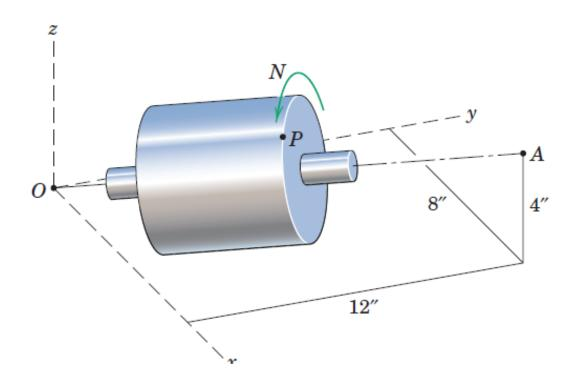
The rotor and shaft are mounted in a clevis which can rotate about the z-axis with an angular  $\Omega$ . With  $\Omega$ =0 and  $\theta$  constant, the rotor has an angular velocity
