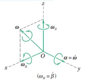
(c) With the position vector of A given by  $\mathbf{r} = 0.693\mathbf{j} + 0.4\mathbf{k}$  m, the velocity of A from Eq. 7/1 becomes
