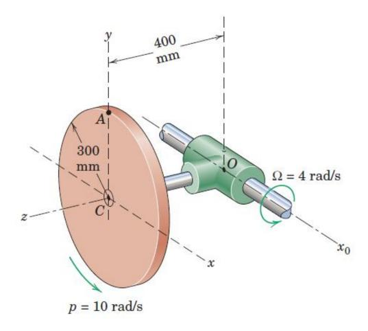
**7/32** If the angular rate p of the disk in Prob. 7/31 is increasing at the rate of 6 rad/s per second and if  $\Omega$  remains constant at 4 rad/s, determine the angular acceleration  $\alpha$  of the disk at the instant when p reaches 10 rad/s.
