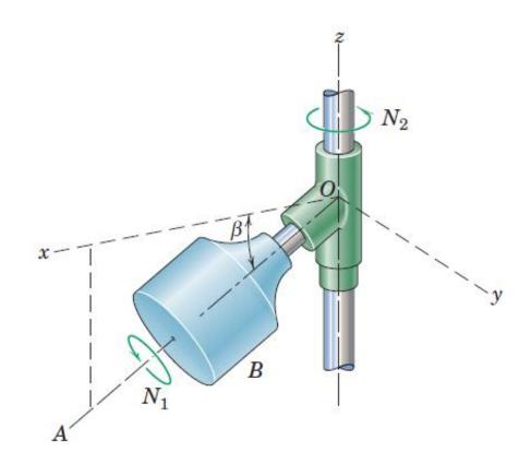
**7/13** The spool A rotates about its axis with an angular velocity of 20 rad/s, first in the sense of  $\omega_a$  and second in the sense of  $\omega_b$ . Simultaneously, the assembly rotates about the vertical axis with an angular velocity  $\omega_1 = 10$  rad/s. Determine the magnitude  $\omega$  of the total angular velocity of the spool and construct the body and space cones for the spool for each case.
