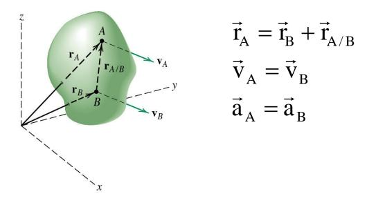
$\vec{r}_{A/B}$  remains constant and therefore its time derivative is zero.
