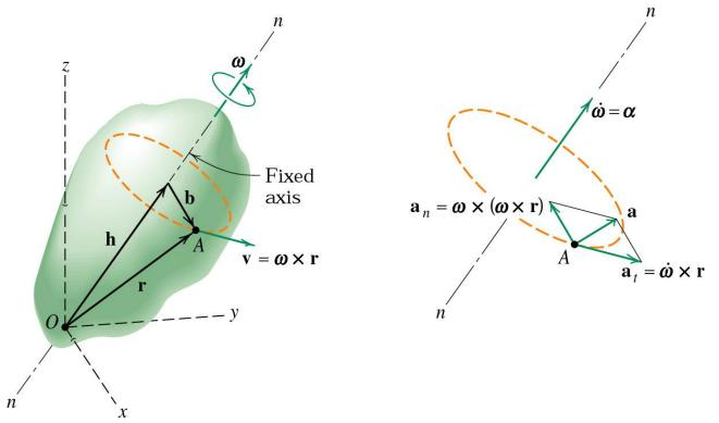
Any point such as A which is not on the axis moves in a circular arc in a plane normal to the axis and has a velocity and an acceleration
