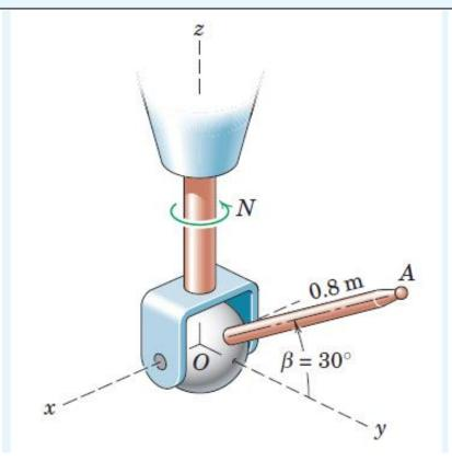
**Solution.** (a) Since the arm *OA* is rotating about both the *x*- and the *z*-axes, it has the components  $\omega_x = \dot{\beta} = 4$  rad/s and  $\omega_z = 2\pi N/60 = 2\pi (60)/60 = 6.28$  rad/s. The angular velocity is
