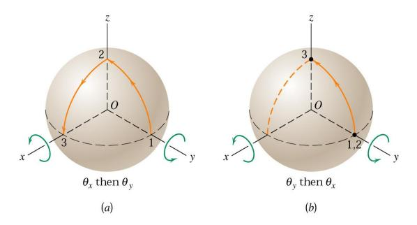
On the other hand, if the order of the rotations is reversed, the point undergoes no motion during the *y*-rotation but moves to point 3 during the 90° rotation about *x*-axis. Thus, the two cases do not produce the same final position, and it is evident from this one special example that finite rotations do not generally obey the parallelogram law of vector addition and are not commutative.  $(a+b\neq b+a)$  Thus, finite rotations may not be treated as proper vectors.
