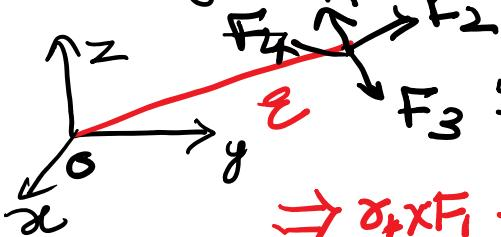
$$\Rightarrow M = M_1 + M_2 + M_3 + M_4 \\ \Rightarrow \sigma_x \times F_1 + \sigma_y \times F_2 + \sigma_z \times F_3 + \sigma_w \times F_4$$
