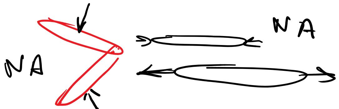
A single force on a single rigid body force on a rigid body is transmissible vector. Line of action play a vital role not the point of application
