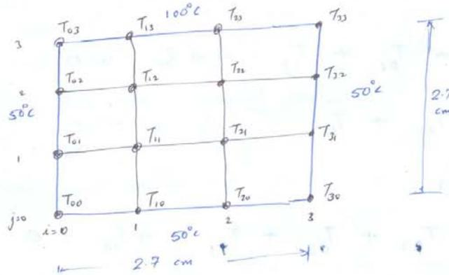
The governing equation is  $\frac{\partial^2 T}{\partial x^2} + \frac{\partial^2 T}{\partial y^2} = 0$
