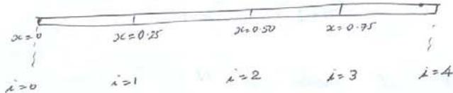
$$\left.\frac{d^2T}{dx^2}\right|_i = \frac{T_{i+1} - 2T_i + T_{i-1}}{\Delta x^2}$$
