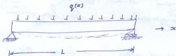
$$EI(x) \frac{d^4 y}{dx^4} = q(x) \quad ; \quad \begin{aligned} y(0) &= 0 \\ y(L) &= 0 \\ y''(0) &= 0 \\ y''(L) &= 0 \end{aligned}$$
