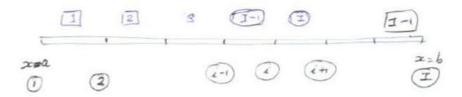
→ The domain is discretised into discrete nodes (1), (2), (3),...,(I) → Again the domain consists of  $\boxed{I-1}$  elements (elements can be linear, quadratic etc.)
