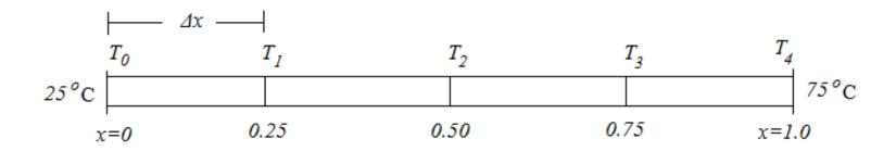
$\Delta x = 0.25$  cm. As per the given data  $T_0 = 25^{\circ}$ C and  $T_4 = 75^{\circ}$ C.  $T_1, T_2, T_3$  are unknowns.
