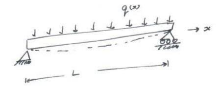
$$EI\frac{d^4y}{dx^4} = q(x); y(0) = 0, y(L) = 0, y''(0) = 0, y''(L) = 0$$
