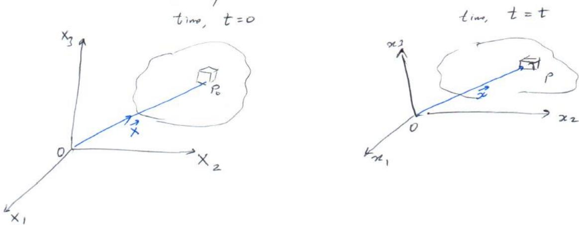
Initially at time  $t=0$ , the position of particle in the continuum  $P_0$  is given by the position vector. The position is represented in material co-ordinates  $O x_1 x_2 x_3$ .
