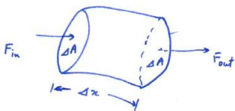
Let the cross sectional area on left be  $= \Delta A = \text{same at right}$ . Only two surfaces allow flux transmission in the control volume.
