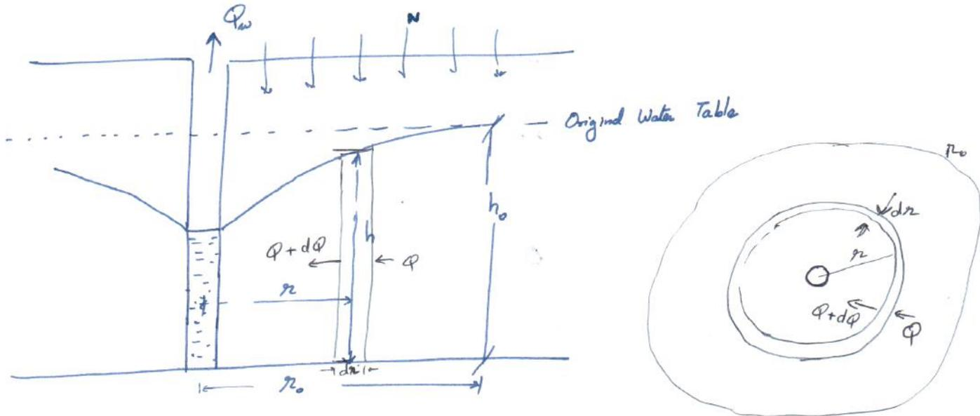
→ For a steady discharge pumping of  $Q_w$  from an unconfined well, to analyse the radial flow into the well.
