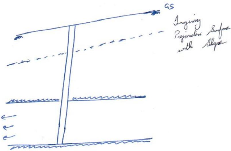
→ The imaginary piezometric surface has a gradient and it is assumed that this gradient is constant. Therefore there will be uniform flow in the confined aquifer.
