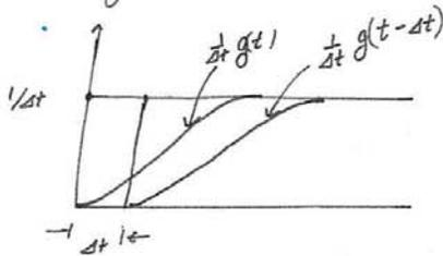
Now from the figure the response of the system for unit pulse input
