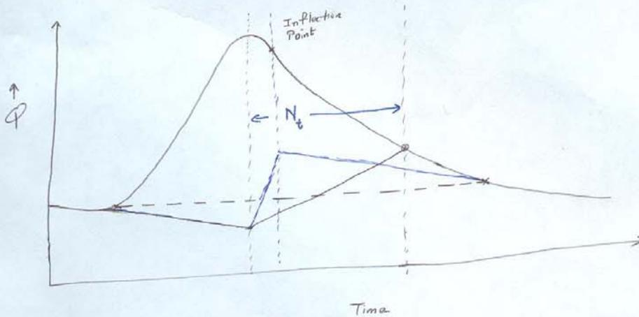
→ The straight - line method - draw a horizontal line from point of beginning of surface runoff to the point where it intersects the receding hydrograph curve.
