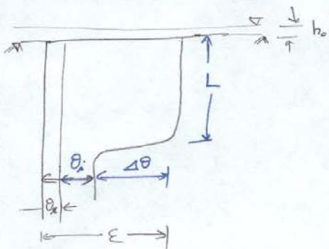
Water is ponded to a small depth  $h_0$  on the soil surface.
