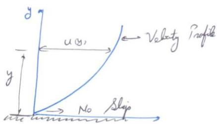
$\left. \begin{array}{l} \text{No-slip in characteristic} \\ \text{of all viscous flows.} \end{array} \right\}$
