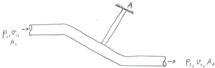
→ ~~The control~~ We were asked to find the torque that has to be resisted by the fixed joint at A due to the fluid motion in the pipe bend.
