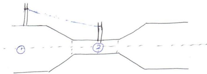
Considering the flow to be steady, frictionless, we can use Bernoulli's principle.
