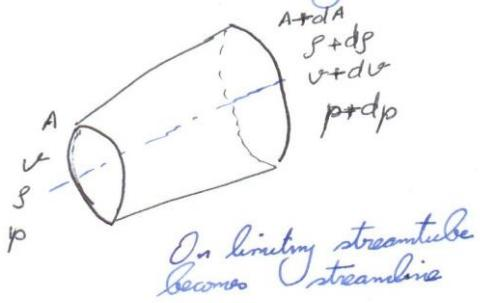
→ The linear momentum equation in the streamwise direction is will be:
