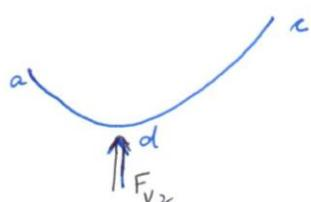
→ The vertical component of hydrostatic force  $F_2$  will be  $F_{V2}$  acting upwards.  ~~$F_b$~~
