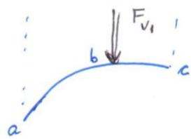
It will have a vertical hydrostatic force component  $F_b$  acting <sup>into</sup> the perpendicular and curved surface.
