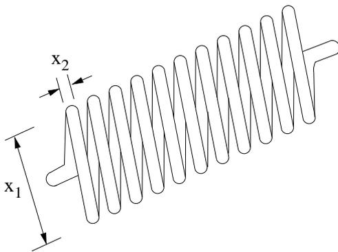
**Figure 13.** A Spring tension/compression example
