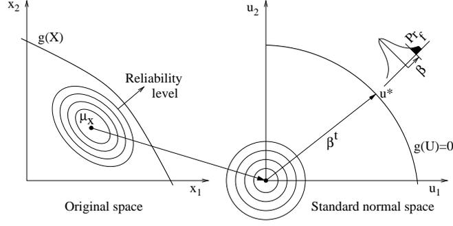
**Figure 1.** Transformation from the original design variable space to the standard normal space.
