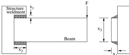
Figure 15. A welded beam structure example
