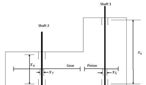
Figure 4: A speed reducer
