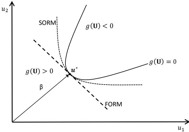
Figure 1: Approximation with FORM and SORM. Here,  $g(\mathbf{U})$  is the limit state function,  $\beta$  is the target reliability, and  $\mathbf{u}^*$  is the MPP
