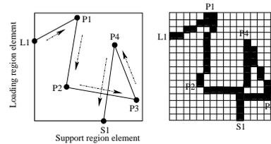
**Fig. 5.** Connectivity between support and loading regions.
