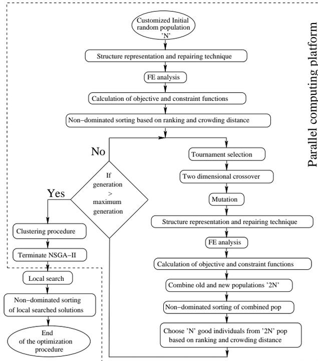
Fig. 3. A flow chart of customized NSGA-II algorithm
