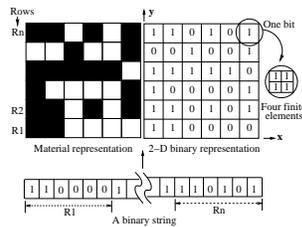
**Fig. 4.** A representation of structure using binary string.
