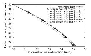
Fig. 9. Prescribed path and path traced by the minimum weight design and local search solutions.
