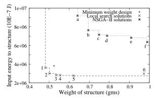
Fig. 8. NSGA-II solutions before and after local search are compared with the single-objective 'minimum-weight' design.
