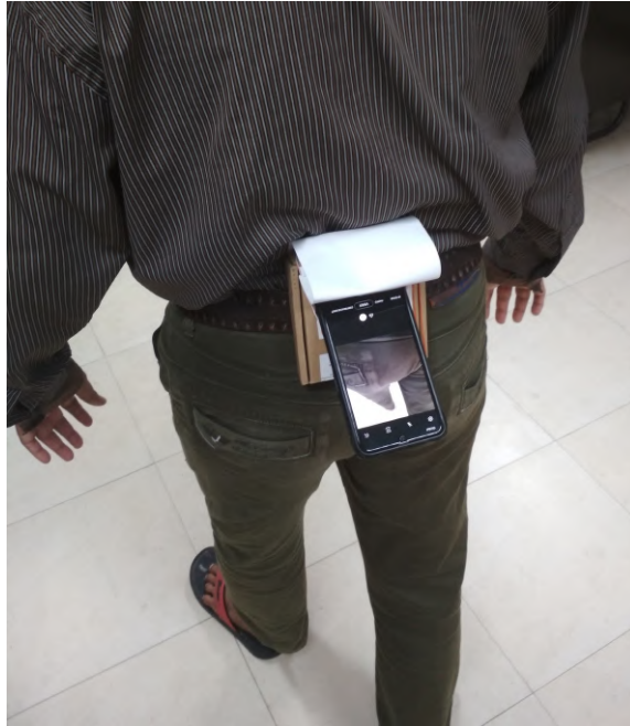
Figure 3.2: Smartphone attached in the back of the user to collect instantaneous frequency for building the model
